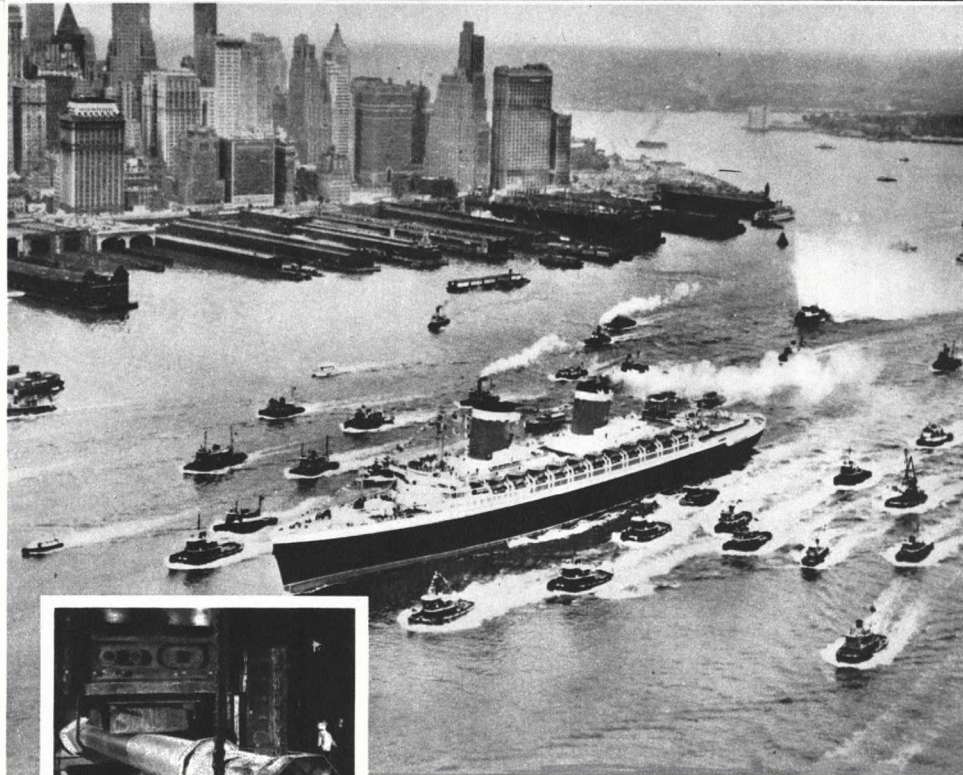
70 MILLION DOLLAR SUPERLINER. On her shake-down cruise, a huge welcoming committee of tugs accompanied the S.S. United States past the New York skyline. U. S. Steel furnished forged steel propulsion shafting which helped establish a new trans-Atlantic speed record. Six of these forged steel shafts were 61 feet long and each weighed 91,500 pounds when it left our mill.
